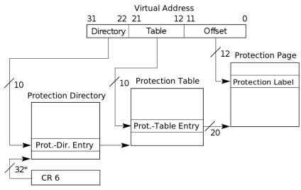
\*32 bits aligned onto a 4-KByte boundary.
