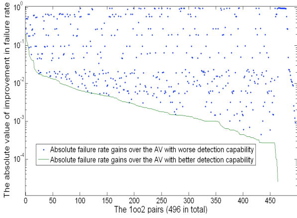
Figure 5. Gains in detection capability (lower failure rates) of a pair of AVs over the individual AVs.
