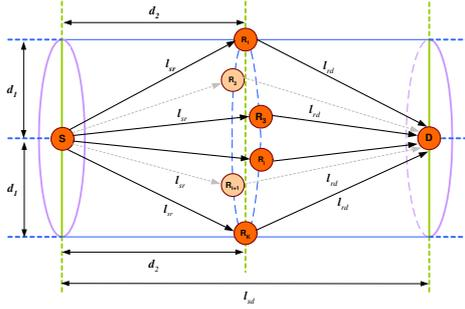
Figure 1: Relay location setup: 3D Parallel Case.
