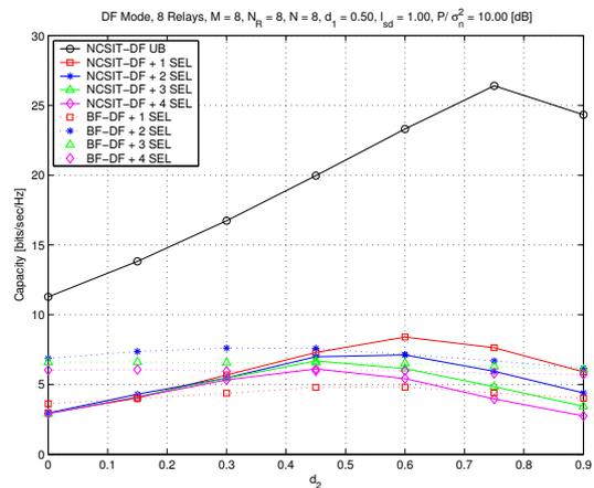
Figure 3: Network capacities for 8 Relays and  $M = N = N_{\mathcal{R}_k} = 8$  for DF Upper Bound, NCSI-DF and BF-DF relaying modes.  $P/\sigma_n^2 = 10$ dB.
