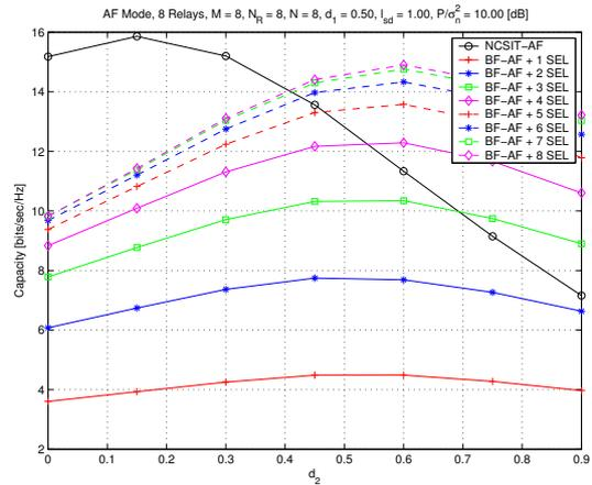
Figure 2: Network capacities for NCSI-AF and incremental relay selection BF-AF modes are given. 8 Relay nodes and  $M = N = N_{\mathcal{R}_k} = 8$ ,  $P/\sigma_n^2 = 10$ dB.
