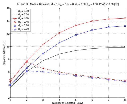
Figure 4: Network capacities for incremental relay selection BF-AF modes are given. 8 Relay nodes and  $M = N = N_{\mathcal{R}_k} = 8$ ,  $P/\sigma_n^2 = 10$ dB.
