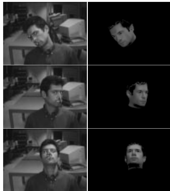
Figure 2. Head rotations supported by the face tracking system, without any marker or specific lighting
