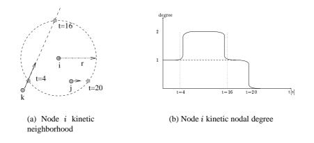
Figure 3: Illustration of nodes kinetic degrees
