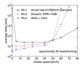
Fig. 5. average delay vs. speed (B = M beamforming)
