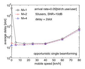
**Fig. 4**. average delay vs. speed (B = 1 beamforming)
