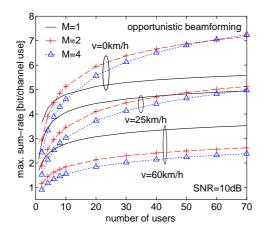
Fig. 2. max sum-rate vs. number of users (beamforming)
