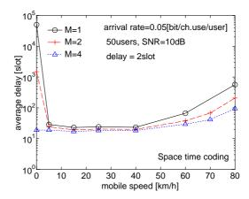
Fig. 3. average delay vs. speed (STC)
