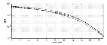
Fig. 2. Scenario 1: SER versus SNR performance of the proposed minimum SER precoder  $-\circ -$ , the trivial precoder -+-, and the minimum PEP precoder  $-\times -$  proposed in [8].
