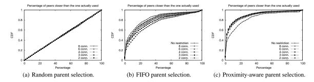
Fig. 7. Percentage of peers in the whole system closer than the one actually used (for those not connected to the source.)
