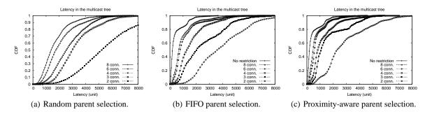
Fig. 9. Latency from root to leaf (in Skitter coordinate units) in the Multicast tree.
