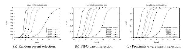
Fig. 8. Level of peers in the multicast tree.
