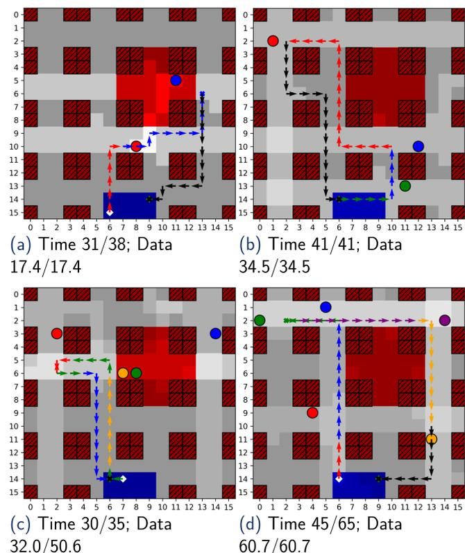
Figure: Illustration of the same agent adapting to differences in device count and device placement as well as flight time limits, showing used and available flying time and collected and available total data in the Manhattan scenario.
