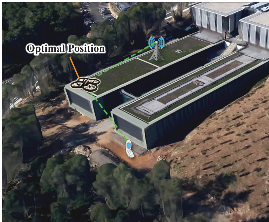
Figure 8.5 – Outdoor experiment setup with UAV relay.
