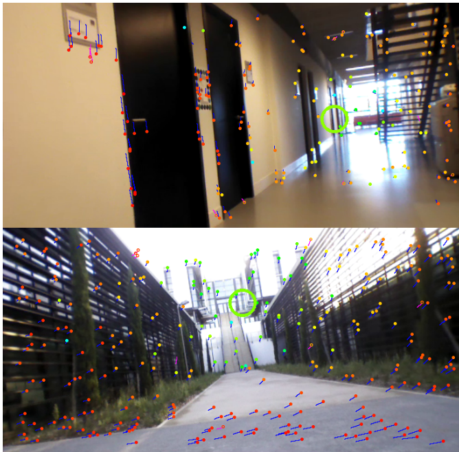
Figure 4. Sparse 3D reconstructions: Blue/purple lines show optical flow vectors consistent/ conflicting with the camera's motion. The points color represents their longitudinal distance – red indicates 1 m and below, cyan for 10 m and above. A larger green circle marks the target flight direction.
