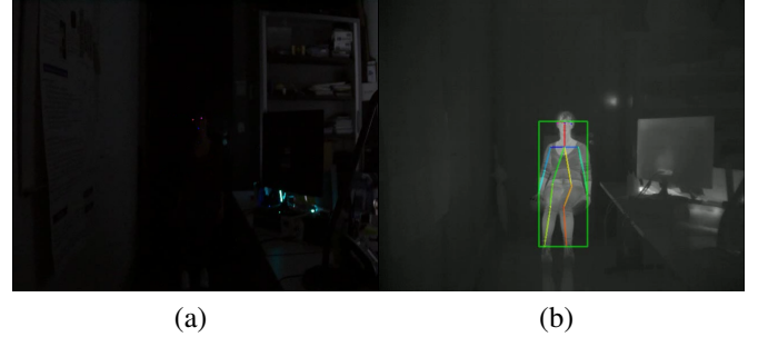
Fig. 1: OpenPose based people detection (a) Visible spectrum (b) Thermal spectrum.
