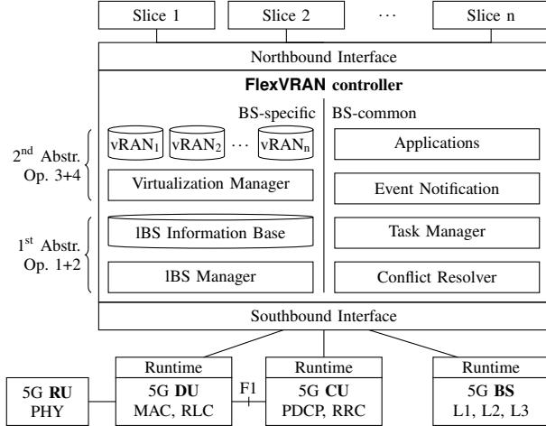
Figure 4. Components and interfaces of FlexVRAN controller.
