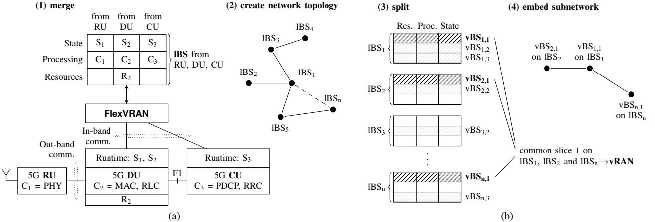
Figure 2. The operations of FlexVRAN to provide the (a) first-level abstraction with operations (1) and (2), and (b) second-level abstractions with operations (3) and (4). Note that the IBS triple in the second-level abstraction only represents customized state, processing, and resources, while common BS functionality remains in the IBS BSD. A missing topological relation between IBSs (dashed line) is present in the virtual sub-network.
