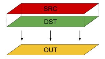
Figure 3: Representation of the Alpha Blending mechanism.
