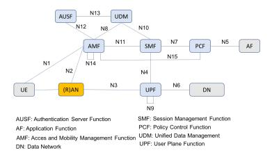
Figure 7: NG core architecture: point-to-point model.
