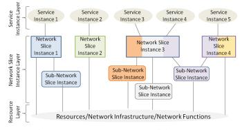
Figure 1: The NGMN network slicing concept.
