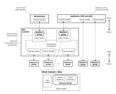
Figure 2: The SDN Architecture for Network Slicing [75].
