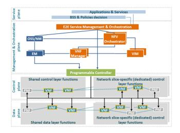
Figure 4: 5GPPP network orchestration architecture [99].
