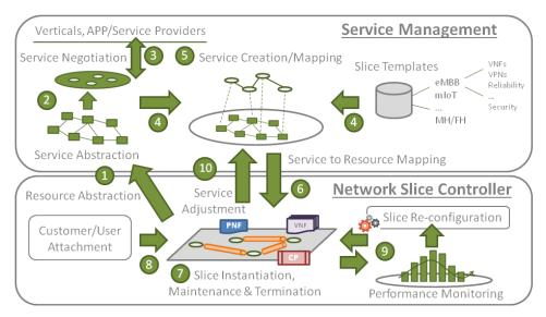
Figure 3: Service management and network slice control.
