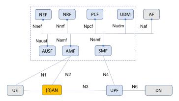
Figure 8: NG core architecture: service-oriented model.
