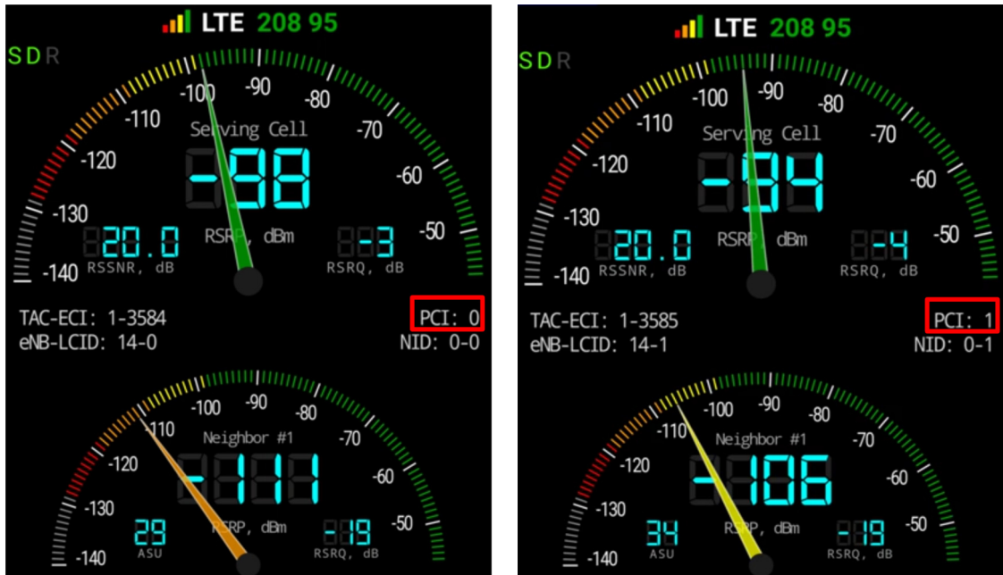
(a) Source/Target eNB RSRP before HO (PCI =0) (b) Source/Target eNB RSRP after HO (PCI =1)
