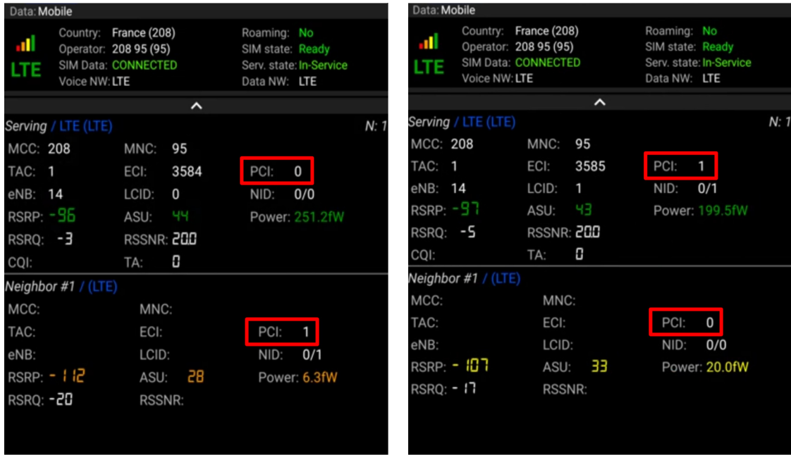
(a) Network information before HO (PCI =0) (b) Network information after HO (PCI =1)
