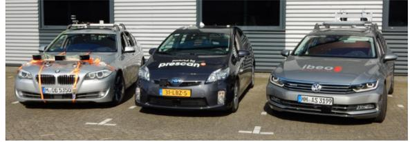
Fig. 4. Test vehicles involved in the first HIGHTS field trials carried out in Helmond: Objective's BMW, TASS's Prius and Ibeo's Passat (left to right).
