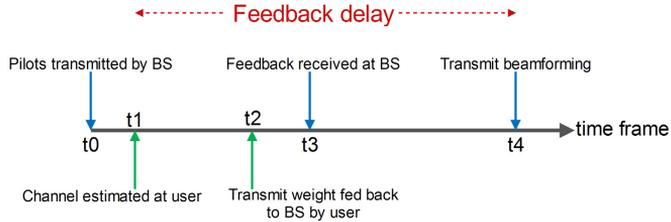
**Figure 3.1.** Feedback Delay Model ©2013 IEEE
