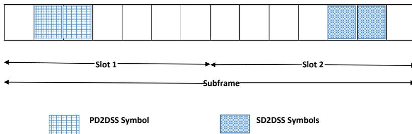
**Figure 4.1.** Synchronization Signals in D2D ©2015 IEEE
