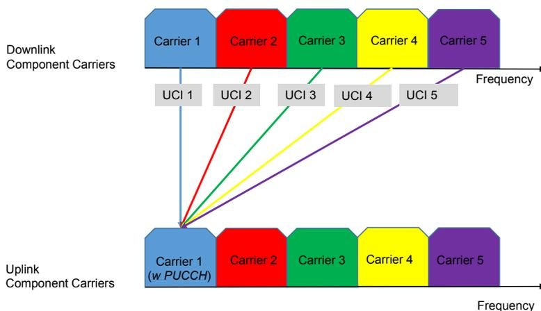
**Figure 5.1.** Example of Combined Uplink Control Information Overhead on Primary Uplink Carrier to Support Downlink Carrier Aggregation for Five Component Carriers ©2016 IEEE
