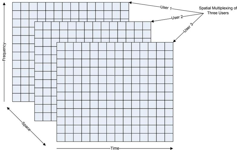
**Figure 2.1.** MU-MIMO: Spatial Multiplexing on Resource Grid
