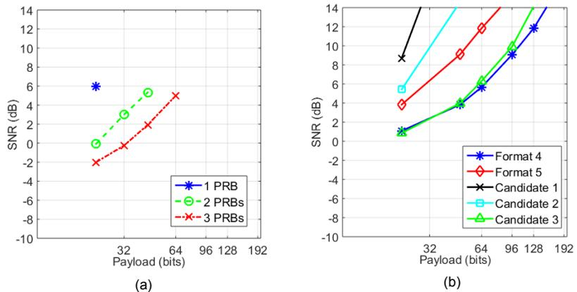
**Figure 5.4.** Required SNR vs Payload for combined target of 1 percent ACK missed detection probability and 0.1 percent NACK-to-ACK error probability (a) PUCCH format 3 compared with similar structure allocated larger bandwidth; (b) New PUCCH formats and other candidates with 1 PRB ©2016 IEEE
