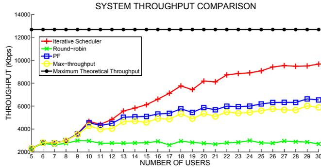
**Figure 6.6.** Throughput Performance for Three-step Iterative Scheduling Algorithm ©2014 IEEE
