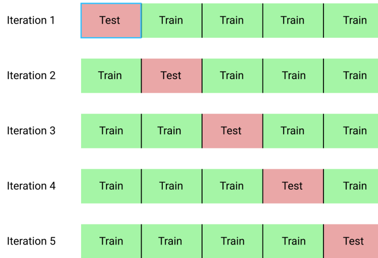
Figure 5: The 5-fold protocol in DCASE development and evaluation set. The split is always done at file level in order to obtain two completely disjoint training and testing sets.
