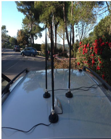
(a) External antennas and GPS receiver
