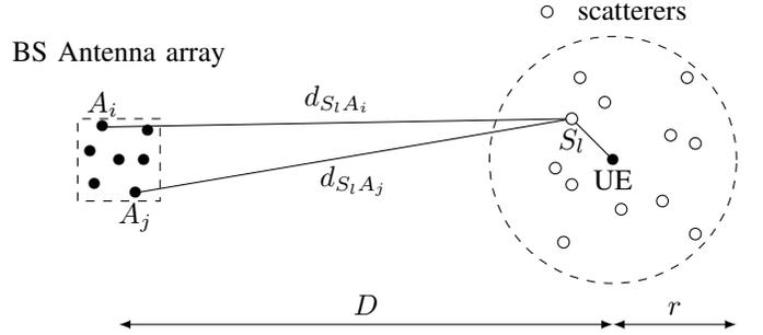
Fig. 2: Illustration of a ray tracing model: the UE antenna is assumed to be surrounded by scatterers randomly located in a ball of radius  $r$  (black and white bullets respectively represent antennas and scatterers).
