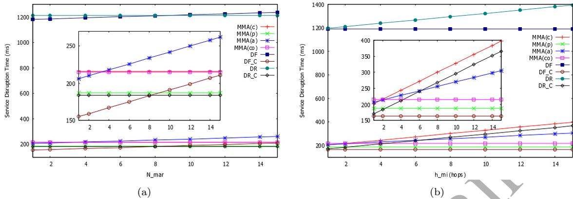
Figure 8: Service disruption as a function of: (a)  $\bar{N}_{mar}$ , (b)  $h_{mi}$ .
