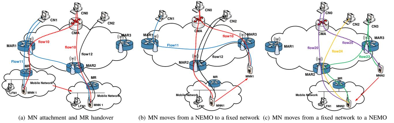
Fig. 1: Architecture and operations of the proposed solution.
