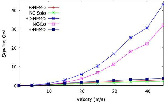
Fig. 8: Signaling cost as a function of velocity ( $v$ ).
