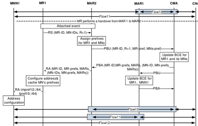
Fig. 4: Signaling flow for MR handover between two MARs.
