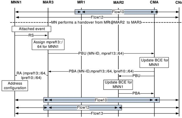
Fig. 5: Handover signaling when an MN moves from a NEMO to an MAR.
