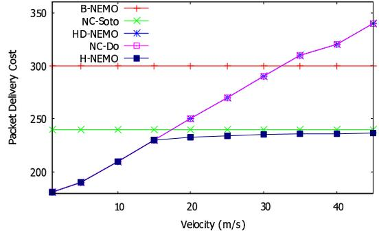
Fig. 9: Packet delivery cost as a function of velocity ( $v$ ).
