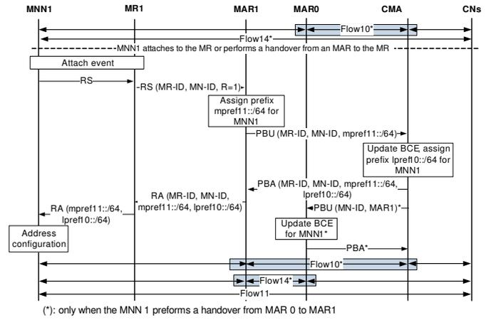
Fig. 3: Initial attachment of the MN.
