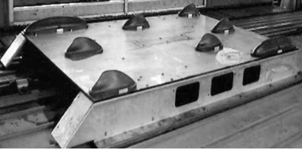
Fig. 6: Antennas on top of the IRIS 320 train.
