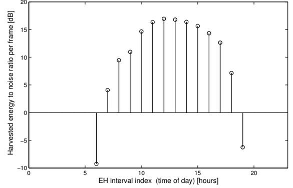
Fig. 3. Model for solar energy harvesting profile.
