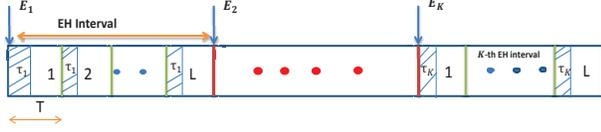
Fig. 2. Energy harvesting time frame structure.
