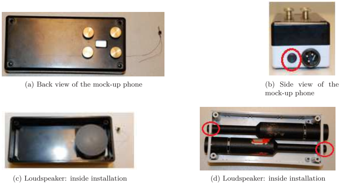
Figure 5.16: Mock-up phone: loudspeaker installation
