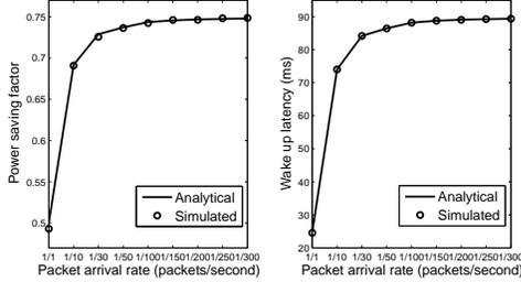
Fig. 3. DRX performance under different packet arrival rates, and  $T_0 = 20ms$ ,  $T_{ON} = 80ms$ ,  $T_S = 160ms$ ,  $N = 16$ ,  $T_L = 320ms$
