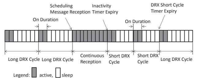
Fig. 1. DRX procedure in LTE
