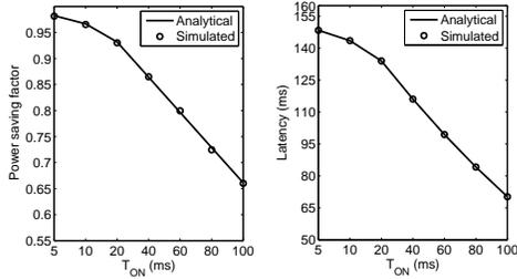
Fig. 5. DRX performance under different On durations, and  $T_0 = 20ms$ ,  $T_S = 160ms$ ,  $N = 16$ ,  $T_L = 320ms$ ,  $\lambda = 1/30$  packets/s.
