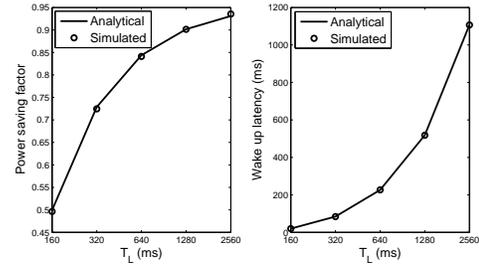
Fig. 8. DRX performance under different long DRX cycle, and  $T_0 = 20ms$ ,  $T_{ON} = 80ms$ ,  $T_S = 160ms$ ,  $N = 16$ ,  $\lambda = 1/30$  packets/s.
