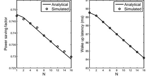
Fig. 7. DRX performance under different DRX short cycle timer, and  $T_0 = 20ms$ ,  $T_{ON} = 80ms$ ,  $T_S = 160ms$ ,  $T_L = 320ms$ ,  $\lambda = 1/30$  packets/s.
