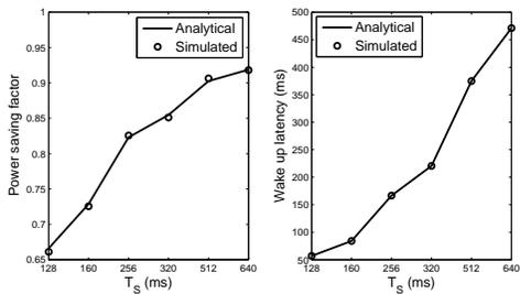
Fig. 6. DRX performance under different short DRX cycle, and  $T_0 = 20ms$ ,  $T_{ON} = 80ms$ ,  $N = 16$ ,  $T_L = 2 \cdot T_S ms$ ,  $\lambda = 1/30$  packets/s.
