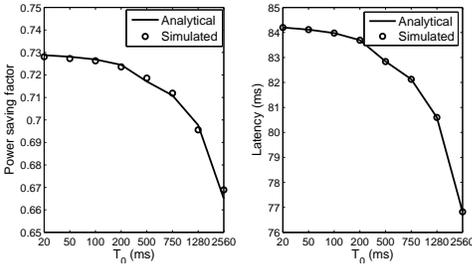
Fig. 4. DRX performance under different inactivity timers, and  $T_{ON} = 80ms$ ,  $T_S = 160ms$ ,  $N = 16$ ,  $T_L = 320ms$ ,  $\lambda = 1/30$  packets/s.
