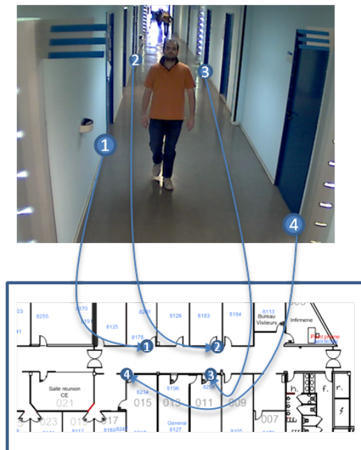
Figure 5.2: The image shows an example of point correspondences needed to compute the homography mapping which allows the transformation from the image space to the map plane. It is important to choose features that are shared between the two modalities.
