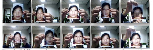
Fig. 3. Different photo-attacks are shown from column (1) to column (5): (1) move the photo horizontally, vertically, back and front; (2) rotate the photo in depth along the vertical axis; (3) the same as (2) but along the horizontal axis; (4) bend the photo inward and outward along the vertical axis; (5) the same as (4) but along the horizontal axis. Fig. is taken from [2].
