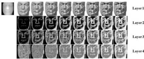
Figure 4: MS-ELBP-DFs of a range face image with different radii from 1 to 8 (from left to right).
