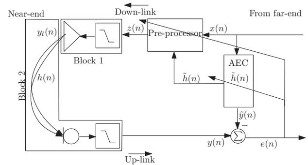
Figure 1: Loudspeaker linearization and acoustic echo cancellation where the LEM is divided into two parts. The first is a nonlinear model and the second is a linear model.
