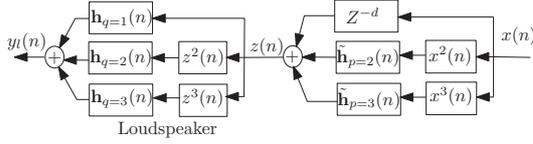
Figure 2: Loudspeaker linearization system.
