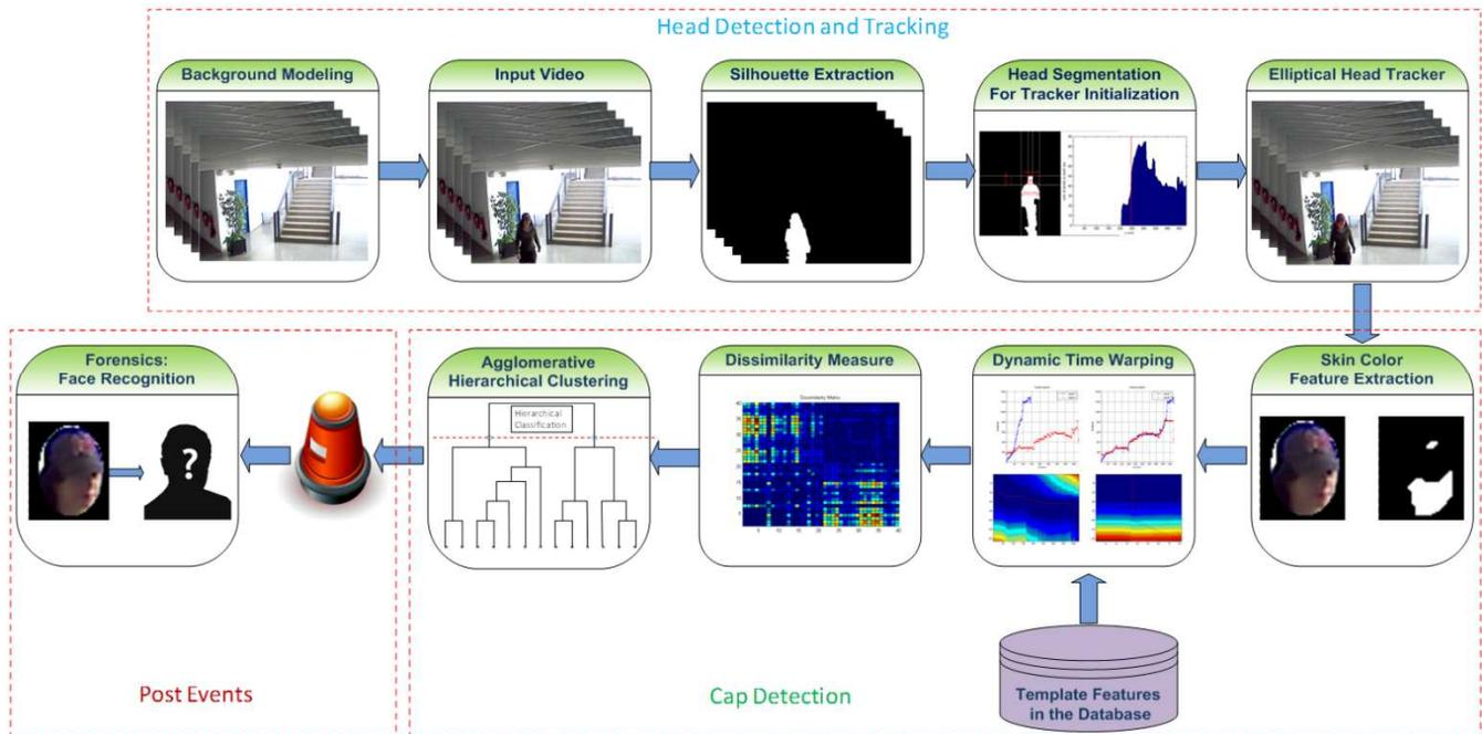
Figure 2. Flowchart of the proposed cap detection system
