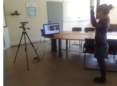
Figure 1: The setup of our demo. A person is standing in front of the sensor triggering the estimation phase by assuming the calibration pose.
