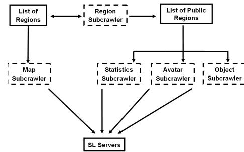
Figure 1: Architecture of the SL crawler
