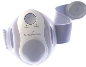
Figure 5.5: Bodymedia Armband : hardware device to measure skin conductance.
