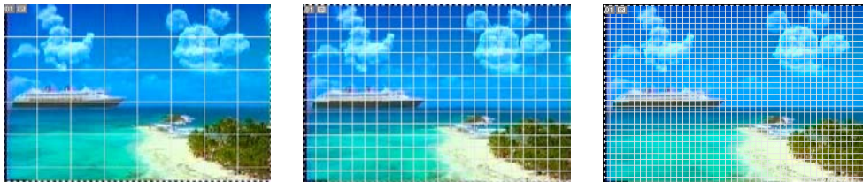
Figure 17. Images decomposed into blocks with different sizes; (a) 44 \times 40 , (b) 16 \times 15 and (c) 8 \times 8 pixels.
