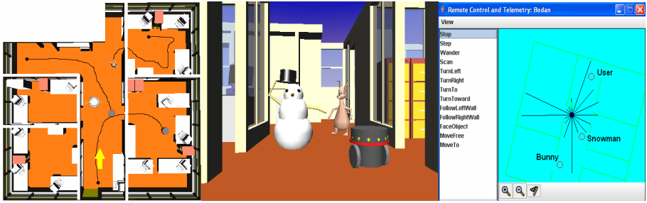
Fig. 4. Views from a Virtual Test Environment. Left: Agent trajectories. Middle: User view. Right: Perspective and tracked objects from Robot Bodan.
