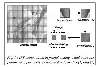
isometric domains (we apply the classical 8 isometries: identity, 4 reflections, 3 rotations). And to allow the domains to be closer from the range, their average brightness and contrast are modified to match those of the range, according to the exact formulas,
