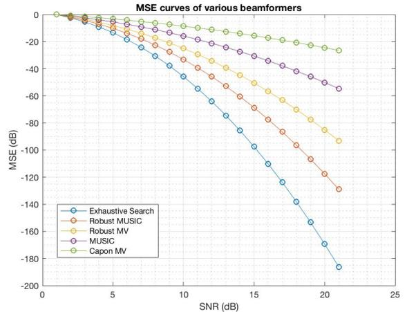
Figure 2: Performance analysis of various beamformers under ellipsoidal uncertainty
