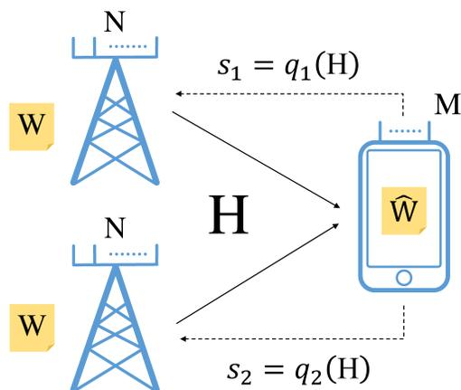
Fig. 1: Illustration of a cooperative MIMO channel with D-CSIT obtained from different error-free feedback links.
