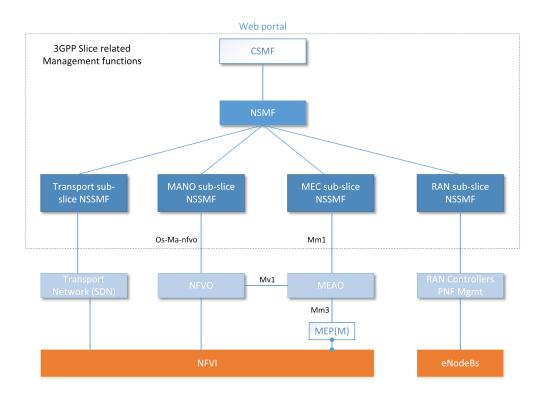
Fig. 4. The proposed Network Slicing orchestration/management architecture, including MEC, in a 5G environment.
