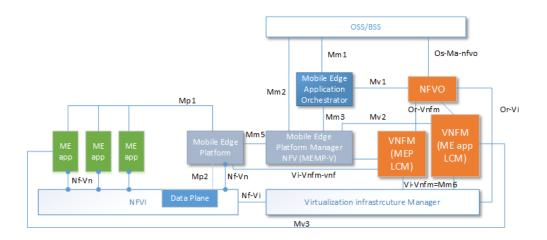
Fig. 2. Updated version of the MEC architecture featuring MEC in NFV (based on [4] and [5]).
