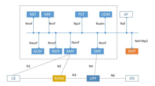
Fig. 3. 5G Core Network service-oriented architecture.
