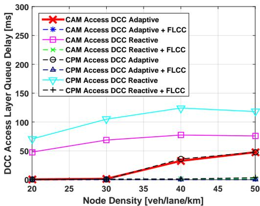
Figure 3: Access DCC Queue Delay, with and without Facilities Layer Congestion Control
