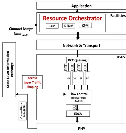
Figure 1: Congestion Control Stack Diagram
