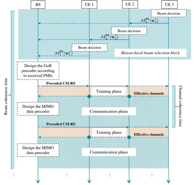
Fig. 2: Signaling sequence of the proposed coordinated beam selection for  $K = 3$ . The beam decision made at each UE leverages the D2D-enabled beam-related information (PMI) coming from higher-ranked UEs in a hierarchical fashion.
