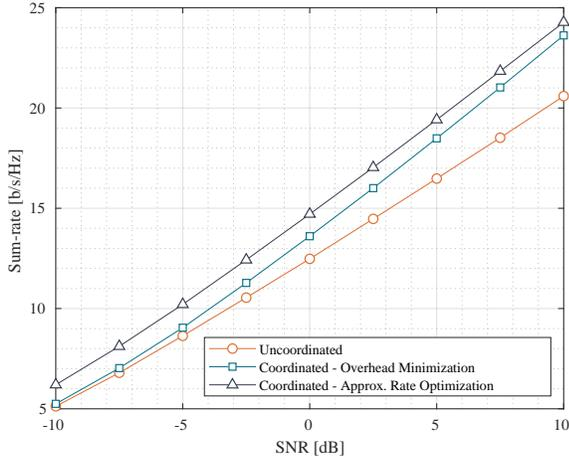
Fig. 3: Sum-rate vs SNR. The channel coherence time is 16 ms. The coordinated algorithms outperform the uncoordinated one.
