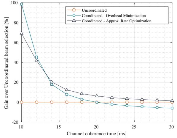
Fig. 4: Gain over uncoordinated beam selection vs channel coherence time. The SNR is 5 dB. Less gains are achieved with the proposed coordinated algorithm as  $T_{\text{coh}}$  increases.
