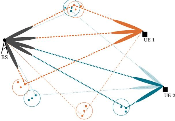
Fig. 1: Scenario example with  $K=2$  UEs. Stronger paths are marked in bold. Uncoordinated SNR-based beam selection results in  $M_{\text{BS}}=5$  beams to train. In this example, UE 2 could instead opt for the non-bold light blue beams to achieve  $M_{\text{BS}}=3$ .
