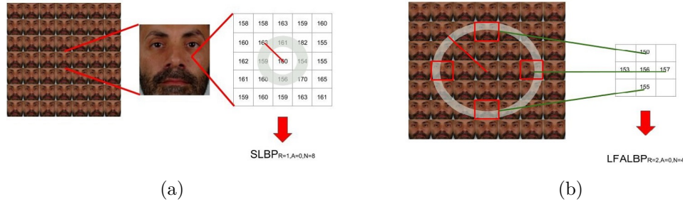
Figure 6.3 – Visual representation of SLBP Figure 6.3a and LFALBP Figure 6.3b used in [148]
