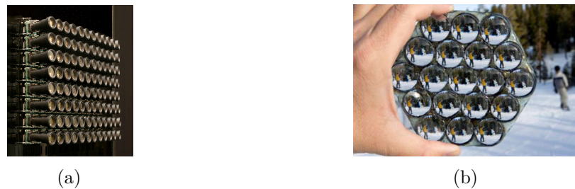
Figure 3.3 – The Stanford multi-camera array (Figure 3.3a) and the Adobe LF camera prototype (Figure 3.3b)
