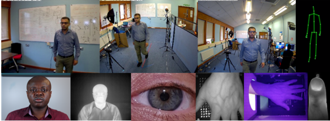
Figure 2.3 – Samples from the PROTECT Multimodal DB database [7]: 2D face, anthropometrics, 3D face, thermal face, iris, hand veins, finger veins.
