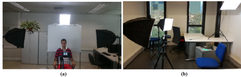
Figure 3.13 – Acquisition environment for LFFD in IST and EURECOM labs.
