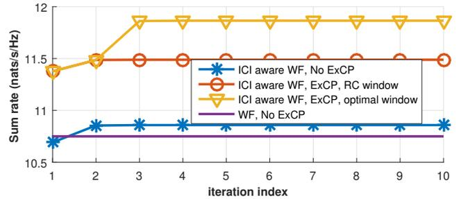
**Fig. 2.** Sum rate comparison with  $N_t = 3, N_r = 3, N = 64, N_e = 16$  at a Doppler of 450Kmph and 20dB SNR.
