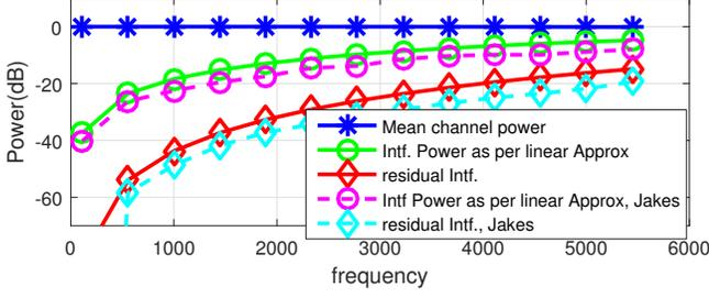
**Fig. 1.** Plot showing the residual error resulting from approximating the channel variation as linear at different Doppler frequencies.
