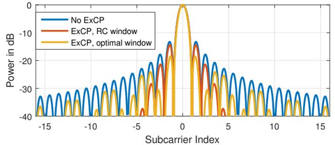
**Fig. 3.** Comparison of windows used to exploit excess CP
