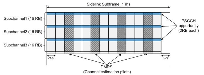
Fig. 1: Sidelink subframe, adjacent PSCCH-PSSCH, 3 subchannels
