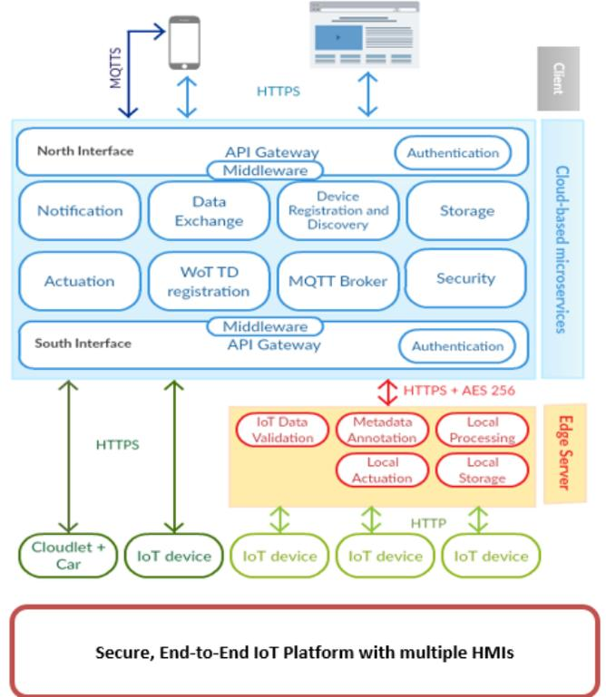
Fig. 1. EURECOM IoT Platform architecture.
