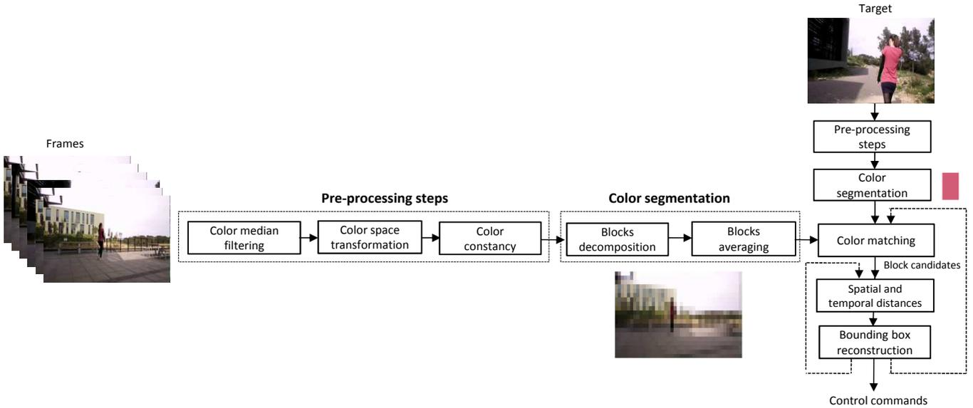
Fig. 1. Flowchart of the proposed color-based detection approach
