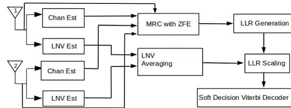
Fig. 5. Schematic of Proposed MLSC for 2 Antenna WiFi Receiver
