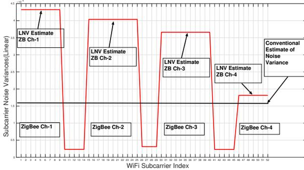
Fig. 4. Conventional Noise variance and Proposed LNV Estimates for 4 Ch-Channel ZigBee Interferers on Single WiFi Channel
