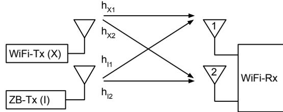
Fig. 2. Signal Model Single Antenna WiFi Transmitter, Single Antenna ZigBee Interferer and Two Antenna WiFi receiver
