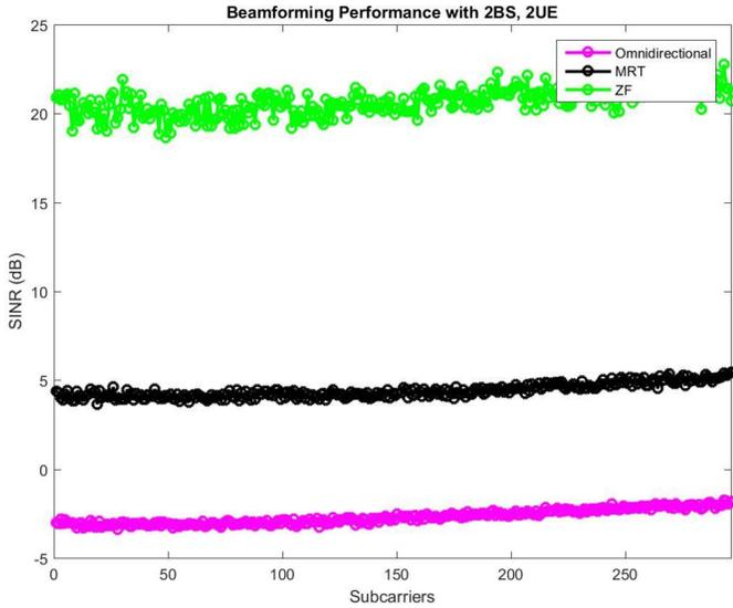
Fig. 4. Performance of MRT and ZF beamformers compared to no beamforming
