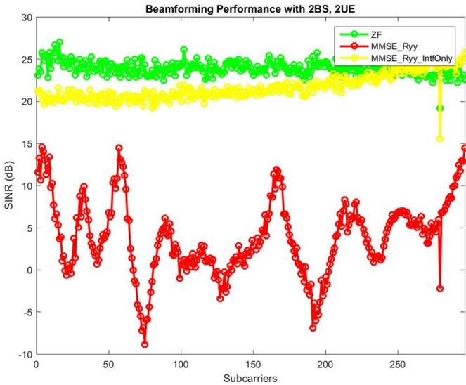
Fig. 5. Comparison of the performance of partial CSIT LMMSE beamformer with that of ZF which requires full information of cross-links.
