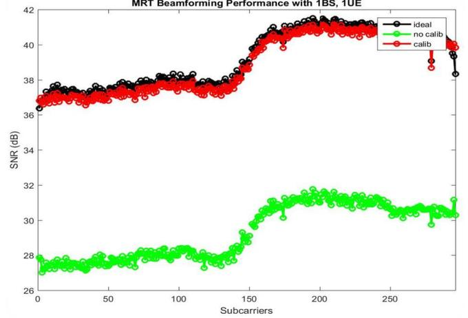
Fig. 3. Performance of MRT with and without calibration for a 23 antenna BS with a single UE.
